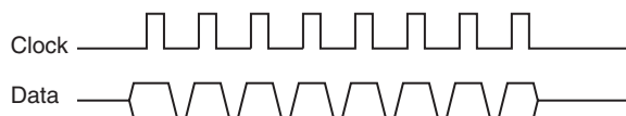
Figure 17.38 Synchronous communications consist of data being latched into the receiver using a clock from the transmitter.
