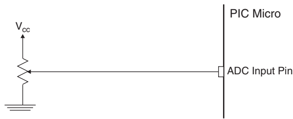
Figure 17.18 A potentiometer wired as a voltage divider can be read using the PIC microcontroller's ADC input.
